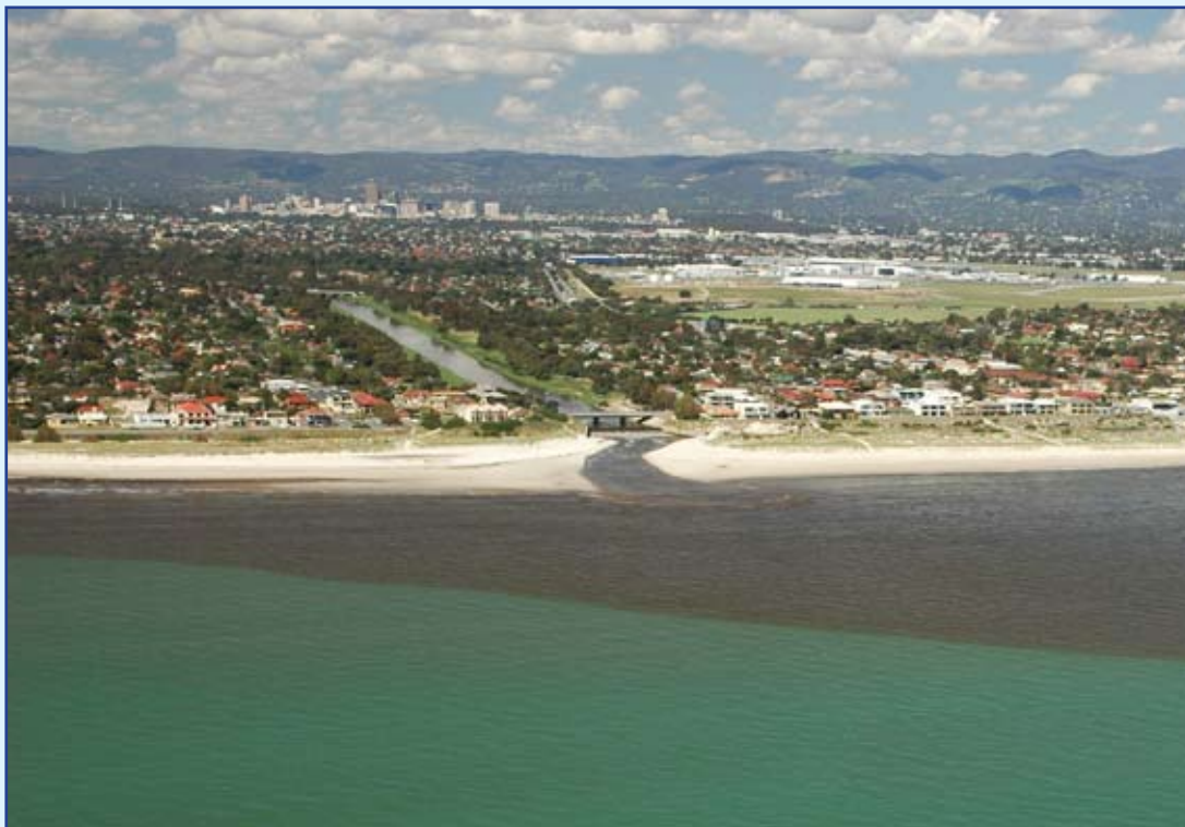
Figure 2: Major discharge of stormwater from the Torrens River into Adelaide's coastal waters on 25 October 2005. Dark region is increased turbidity. Photo: S. Bryars
